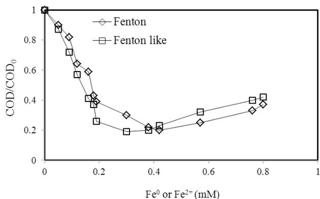
Fig. 4. Effect of Fe<sup>0</sup> or Fe<sup>2+</sup> on COD removal efficiencies obtained for Azithromycin antibiotic by Fenton and Fenton-like processes (conditions: initial antibiotic concentration, 100 mg L<sup>-1</sup>; H<sub>2</sub>O<sub>2</sub> concentration, optimum dosage; reaction time, 60 min).
