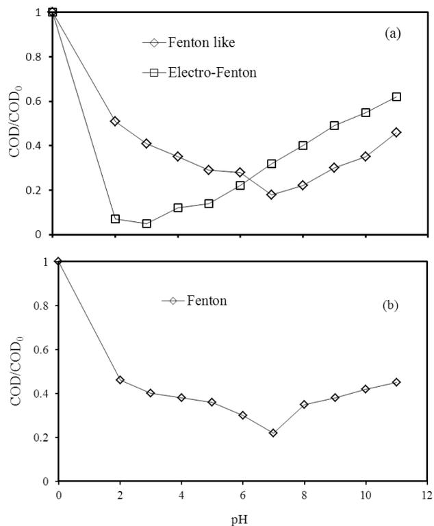
Fig. 2. Effect of pH on COD removal efficiencies obtained for Azithromycin antibiotic by Fenton like and Electro-Fenton (a), Fenton (b) processes (conditions: initial antibiotic concentration,  $100 \text{ mg L}^{-1}$ ;  $\text{H}_2\text{O}_2$  concentration,  $0.1 \text{ mM}$ ;  $\text{Fe}^0$  or  $\text{Fe}^{2+}$  concentration,  $0.1 \text{ mM}$ ; current density,  $20 \text{ mA cm}^{-2}$ ; reaction time, 60 min).
