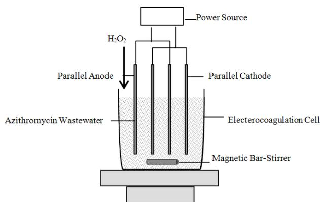
Fig. 1. A schematic diagram of the electrochemical reactor.
