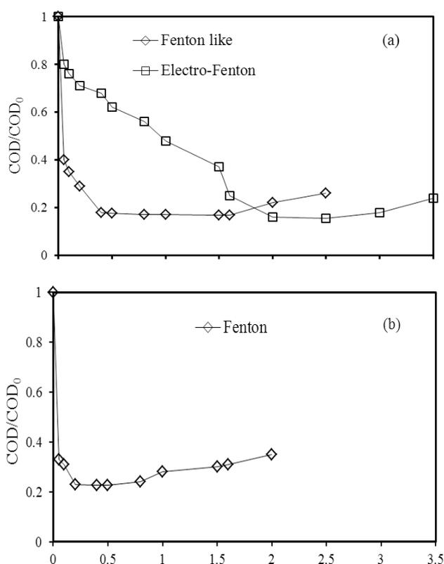
Fig. 3. Effect of  $H_2O_2$  on COD removal efficiencies obtained for Azithromycin antibiotic by Fenton-like and Electro-Fenton (a), Fenton (b) processes (conditions: initial antibiotic concentration, 100 mg L<sup>-1</sup>;  $Fe^0$  or  $Fe^{2+}$  concentration, 0.1 mM; current density, 20 mA cm<sup>-2</sup>; reaction time, 60 min).
