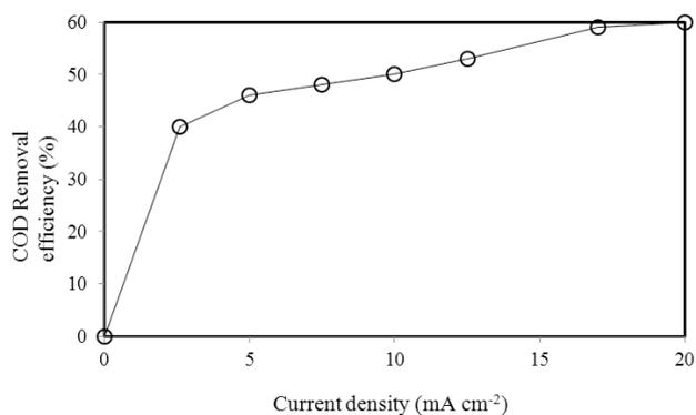
Fig. 5. Effect of current density on COD removal (initial antibiotic concentration, 100 mg L<sup>-1</sup>; reaction time, 30 min; pH, 3.0; H<sub>2</sub>O<sub>2</sub>, 2 mM; initial conductivity, 390 μS cm<sup>-1</sup>; distance between plates, 20 mm).
