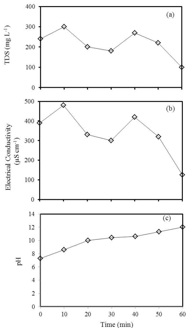
Fig. 6. Change in the characteristics of the solution (a) total dissolved solids, (b) electrical conductivity (c) pH (current density, 20 mA cm<sup>-2</sup>; initial conductivity, 390 μS cm<sup>-1</sup>; distance between plates, 20 mm).
